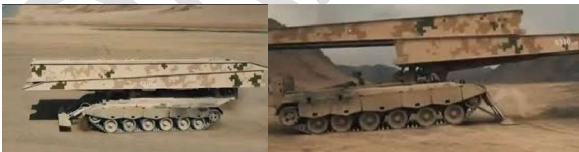
Figure 5.12 GQL-410 AVLB At manoeuvre and deploying
