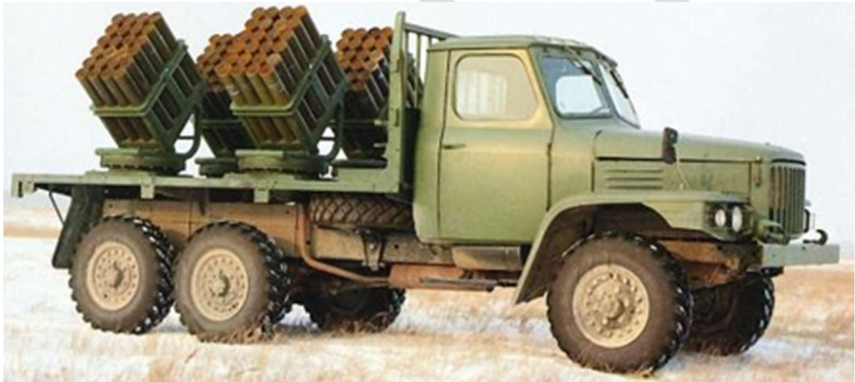
Figure 4.1 GBL-132 Mine Laying vehicle
