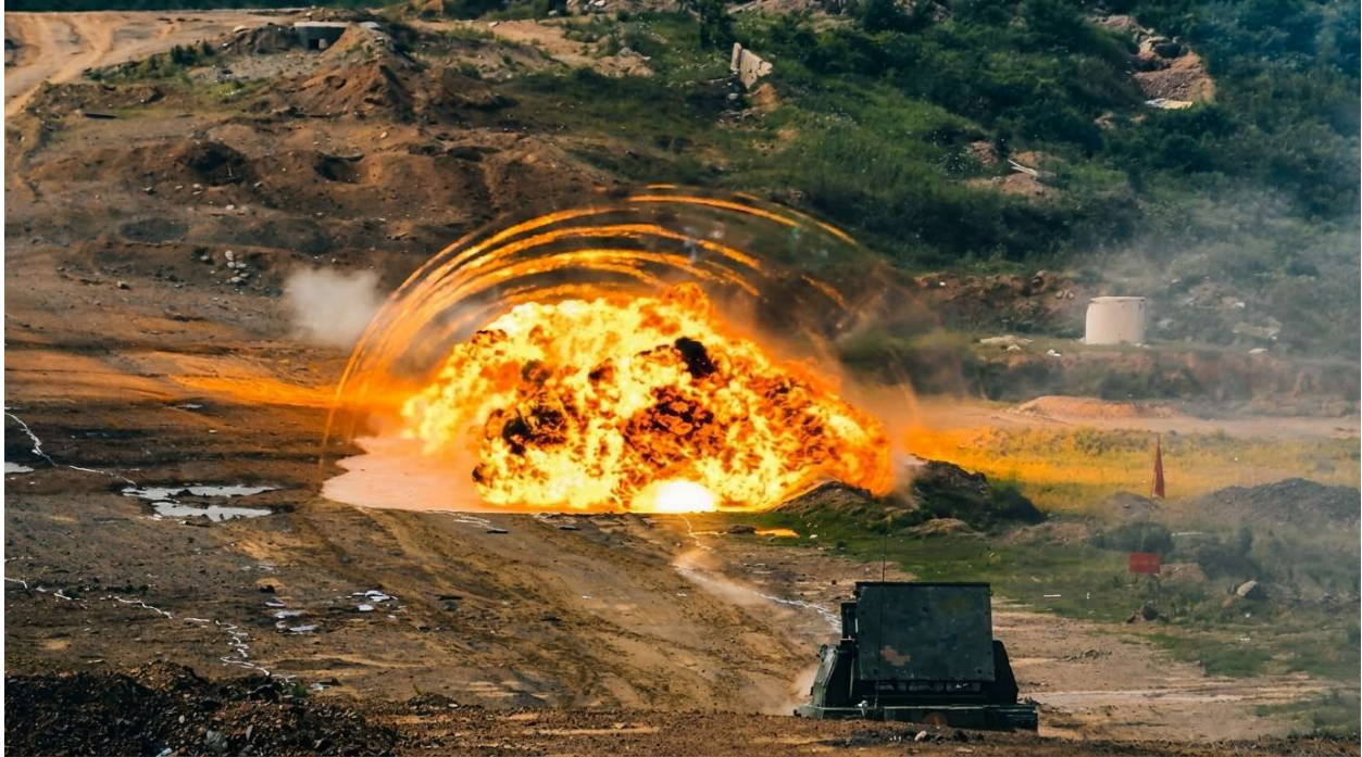
Figure 5.3 – GSL-133 detonates its line charge
