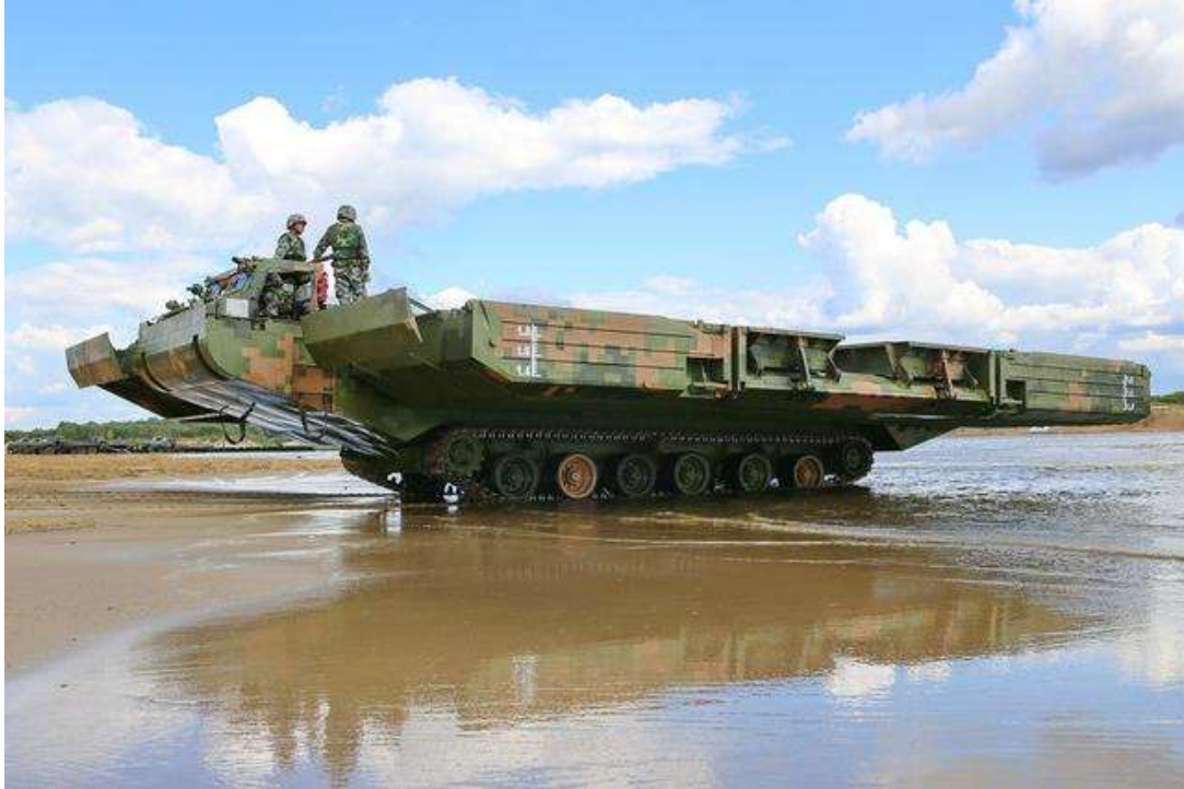
Figure 4.4 GZM-003 Ferry and Floating Bridge
