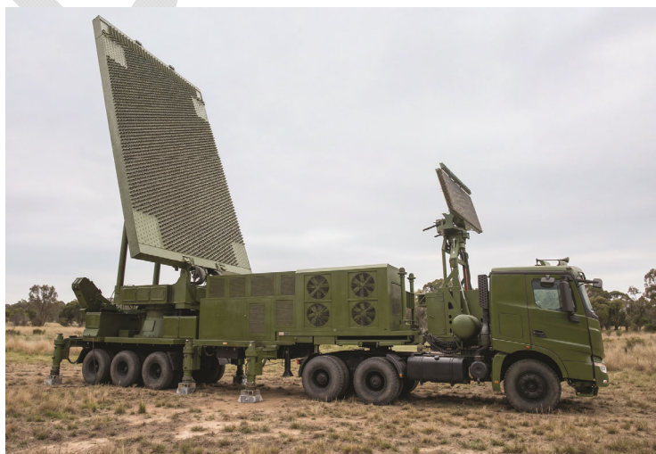
Figure 2C.3 – SLC-7 Long Range Surveillance Radar
