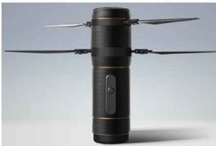
Figure 5.3: Example of a coaxial dual rotor uncrewed aircraft system
