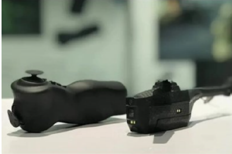
Figure 5.2: Example of a mono-rotor uncrewed aircraft system, a 'nano' drone
