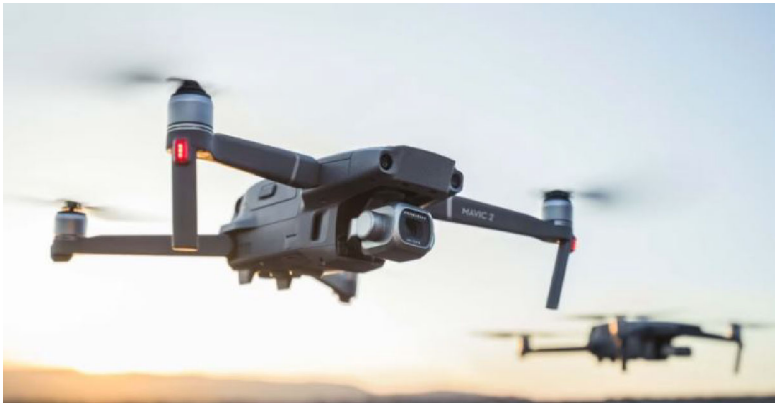
Figure 2.7: DJI Mavic 3 – typical quadcopter
