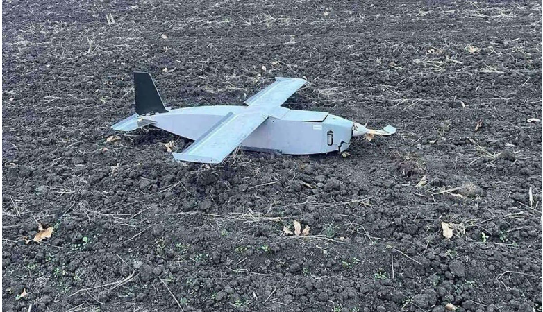
Figure 4.11: Unarmed Russian deception drone with high radar cross section intended to activate A2AD radars and deplete Ukrainian ammunition stores
