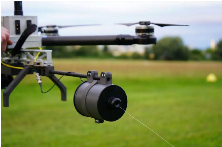
Figure 7.13: Fibre optic cable reel on a fly-by-wire controlled drone in Ukraine 2024
