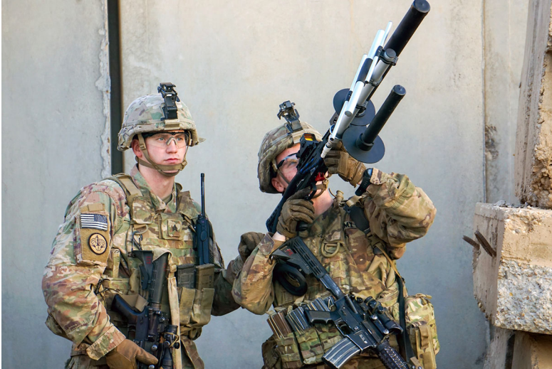
Figure 7.2: Soviet LPD 820 electronic countermeasures anti drone rifle – operates at 2.4 GHz and 5.8 GHz
