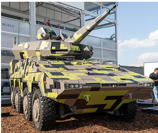
Figure 7.10: Rheinmettal Skyranger 30 anti-uncrewed aircraft system
