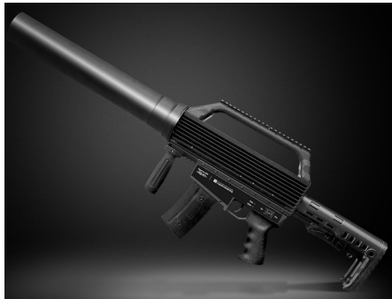
Figure 7.2: Soviet LPD 820 electronic countermeasures anti drone rifle – operates at 2.4 GHz and 5.8 GHz
