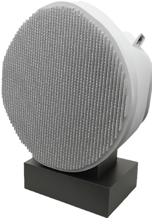
Figure 9.3: United States AN APG-77 Active Electronically Scanned Array
