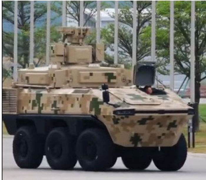
Figure 7.4: A laser-based counter drone system mounted on a 6×6 IFV base
