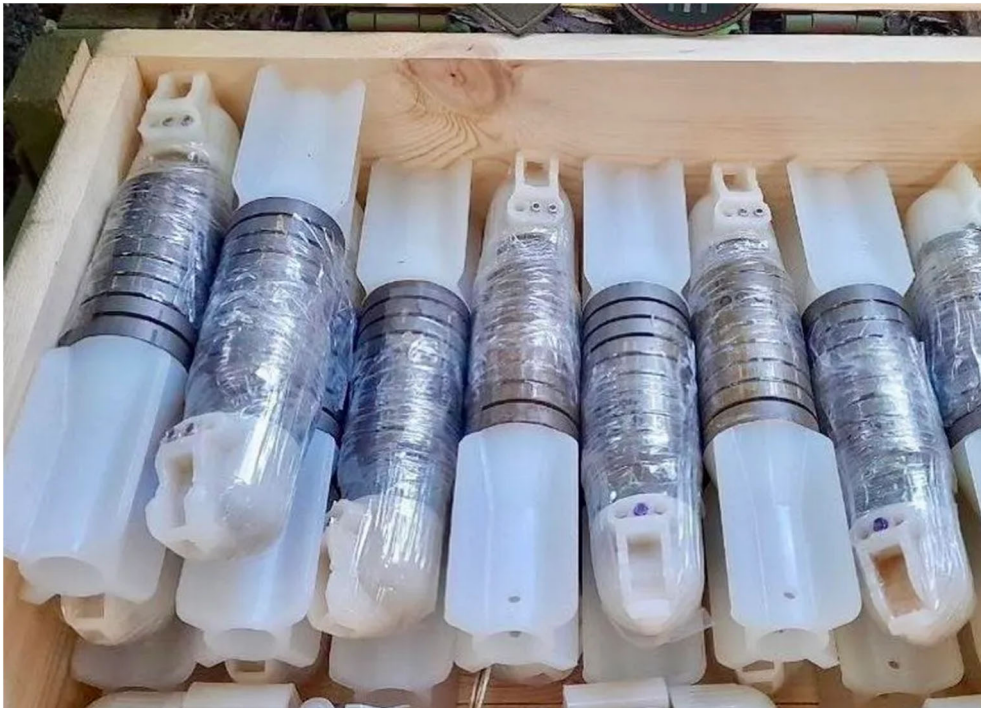
Figure 4.4: Soviet manufactured drone bombs – using steel rings, PVC moulded stabilising fins and protective fuse cap
