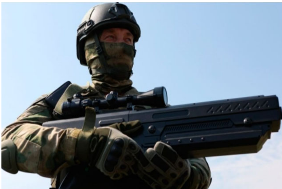
Figure 7.2: Soviet LPD 820 ECM Anti Drone Rifle – operates at 2.4 GHz & 5.8 GHz
