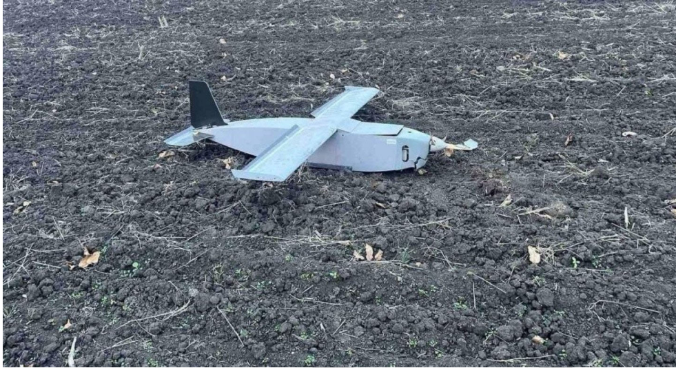
Figure 4.11: Unarmed Russian deception drone with high radar cross section intended to activate A2AD radars and deplete Ukrainian ammunition stores
