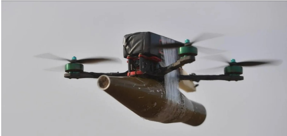
Figure 2.8: FPV drone with an RPG warhead
