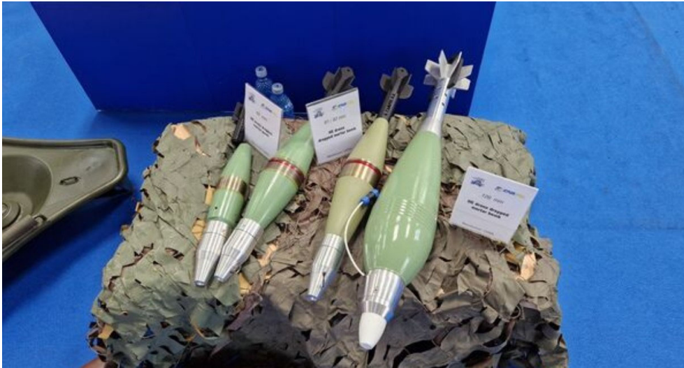
Figure 4.6: Romanian drone-dropped munitions (L-R: 60 mm, 81 mm, 82 mm, and 120 mm), showing the polymer fins on the smaller calibres to reduce weight
