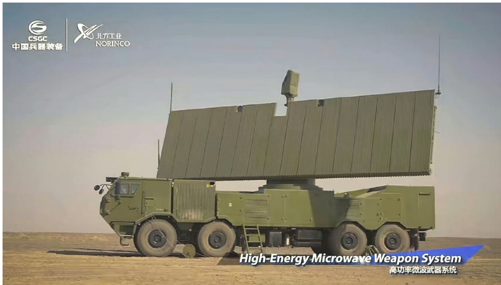
Figure 7.6: Microwave planar array mounted on an 8×8 truck chassis. Note the smaller tracking radar plate on the top centre of the larger microwave plate
