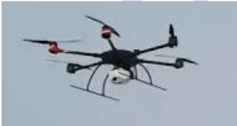
Figure 2.9: Prototype maritime surveillance hexacopter (six rotors) drone with flying time of 75 min
